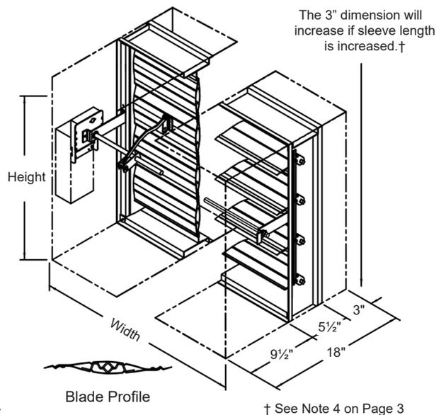
Combination Fire/Smoke Damper • 3 Hr. Rated • Airfoil Blade • Leakage Class I • 250°F or 350°F Rated • Galvanized Steel
